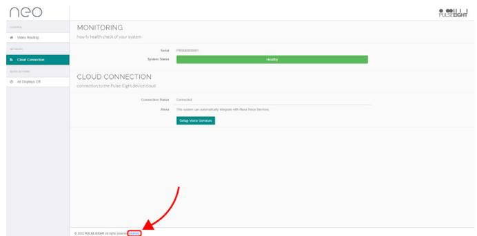
When setting up the matrix, it is important that the installer can access the admin menu on the Web Interface to configure the matrix according to the installation's requirements. This is accessed by clicking the Admin hyperlink and entering 'admin' in the password on first install.
