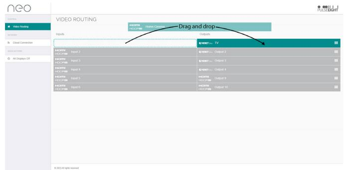
The front page of the web interface features a user-friendly drag and drop for video routing and display showing all available inputs and outputs.
