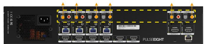
If you wish to use the audio outputs from the matrix, please connect cables to the relevant output. There are 6 output zones, where each zone features Optical and Digital Coax options that can work simultaneously.
