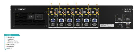
If you wish to use the breakout audio outputs from the matrix, please connect cables to the relevant output. There are 6 output zones, where each zone features Optical and Digital Coax options that can work simultaneously.
