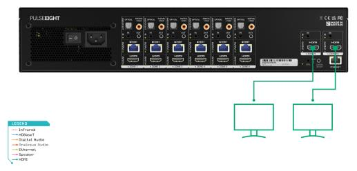
For Output ports 9 and 10, connect sink devices (e.g. TVs) directly via high speed HDMI® cables.
