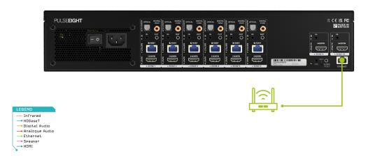
It is necessary to connect a standard Ethernet cable (Category 5e/6/7) from the matrix's 'Ethernet' port to your router or network switch. Crossover cables are not supported.
