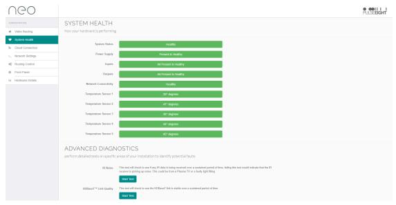
Under the System Health tab, information about the hardware's performance is displayed. The colour-coded (Green = Good, Orange = Warning, Red = Issue) boxes will indicate if it is performing correctly along with the reading of the internal temperature sensor that will indicate if the system is overheating.
