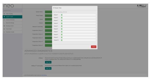
The IR Noise Test will check to see if any unwanted IR noise is being received over a sustained period of time for each port. Failing this test would indicate that the IR receiver on its video output zone (neo receiver) is picking up noise in its environment.
