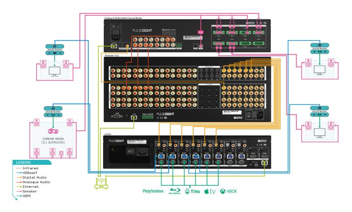
This is an example of a wiring diagram of the neo:8a with a dedicated audio matrix switch (e.g. ProAudio1632) and an amplifier (e.g. ProAmp8).
