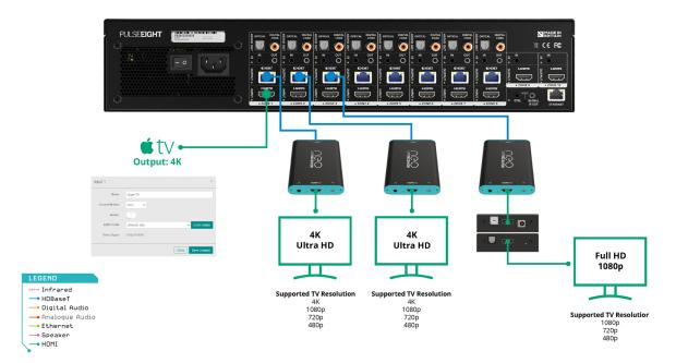
When this occurs, it is possible to use a separate 4K Downscaler (e.g. P8-HDMI2-SP2-DS) which ensures that all displays receive the maximum resolution possible.
