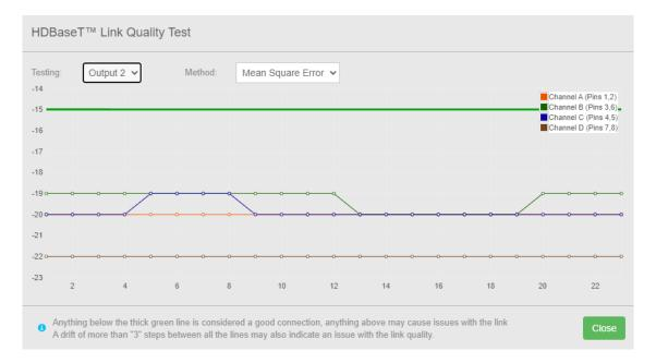
The HDBaseT Link Quality Test will check the HDBaseT link is stable over a sustained period of time. There are two drop down menus, the first is the output you are testing, the second is the type of test you are doing.
