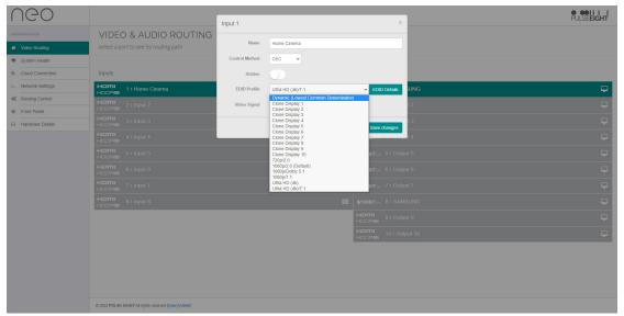
The matrix does not support individual video downscaling. If there is a mixture of displays with different resolution capabilities, then it is important to select the correct EDID profile and/or use an external downscaler.
